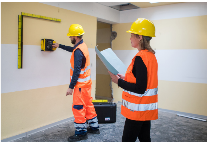
Real-time investigation of concrete structures is fast and simple with C-thrue: visualize on-site results directly on the multi-touch display.
