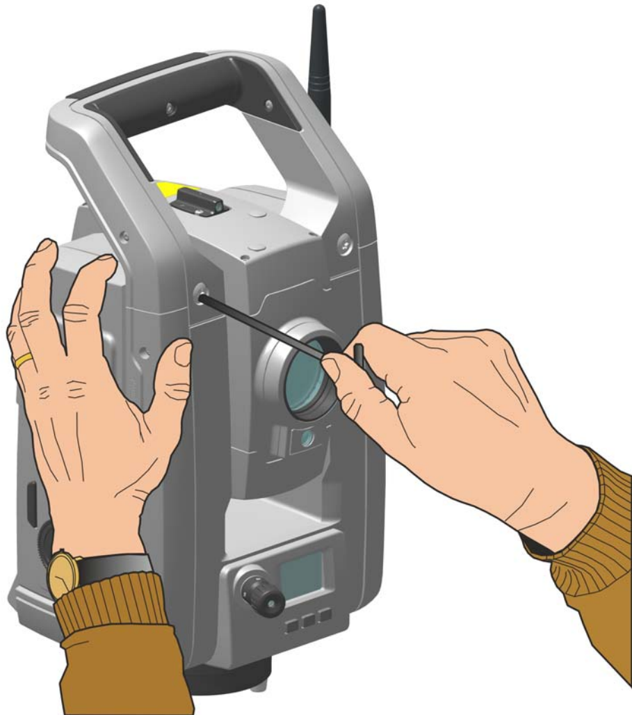
Figure 2.13 Removing the instrument handle
