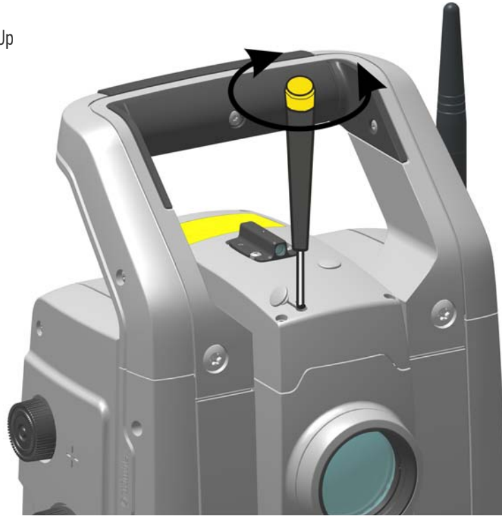
Figure 3.7 Laser pointer vertical position adjustment
